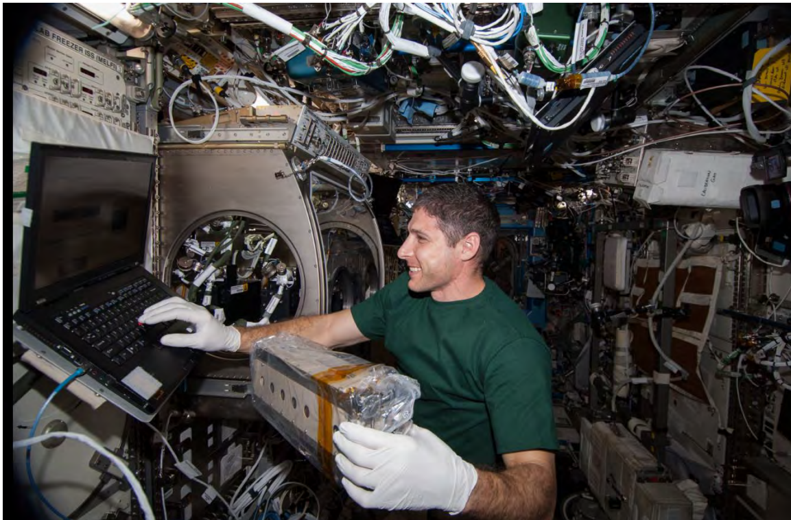
The astronaut Mike Hopkins installs the DCMIX-2 cell array into the Selectable Optical Diagnostic Instrument (SODI) on-board the ISS on 30 November 2013 ( Credit: NASA ).
