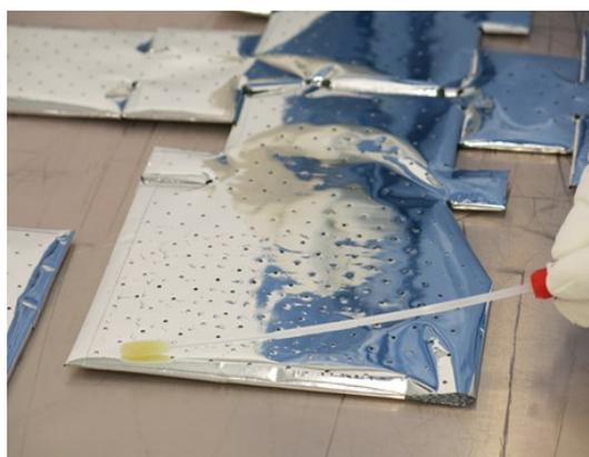
Figure 44 – Bioburden assay sampling using a swab (credit: TAS)
