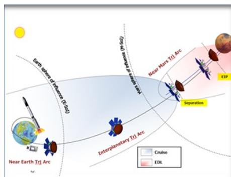
Figure 42 – Interplanetary transfer for ExoMars 2020 mission (credit: TAS)
