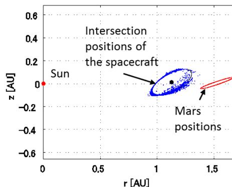
Figure 33 - Example of intersection points on Mars B-plane.
