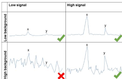
Figure 19 – Signal to background noise ratios, to detect compounds *x* and *y* they must be present at significantly higher quantities than the background. To reduce the background, and therefore increase the sensitivity of the instrument, we must have less contamination.
