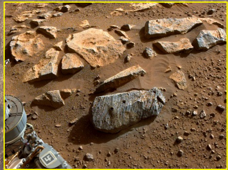
"Rochette" After Perseverance Sampling: Sept 7, 2021, PDT, shows two holes where the rover's drill obtained chalk-size samples from rock nicknamed "Rochette." Credits: NASA/JPL-Caltech.
