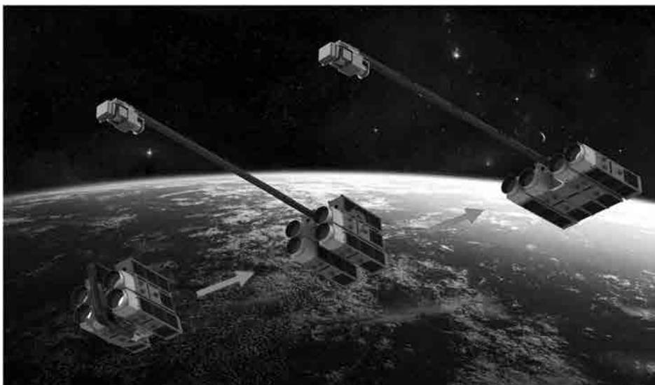
Fig. 2. 4 Concept of the Autonomous Assembly of a Reconfigurable Space Telescope (AAReST) mission consisting of an arrangement of 10 cm diameter circular mirrors attached to a cluster of CubeSats. Image Credit: AAReST Team, California Institute of Technology ( http://www.pellegrino.caltech.edu/aarest1/ )
