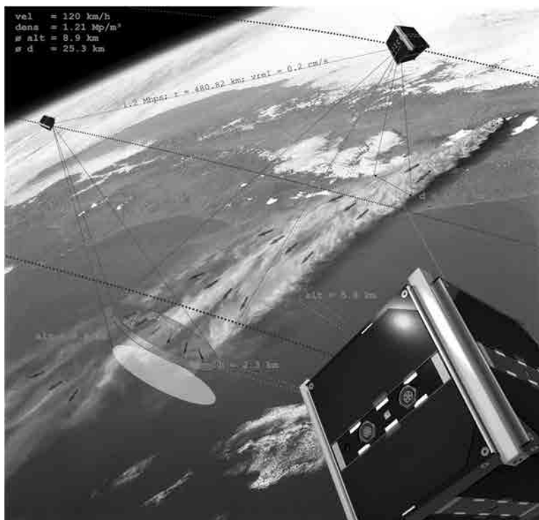
Fig.3.6 The three TIM satellites focus on the same target area for 3D-imaging by photogrammetric methods. Image Credit: Zentrum für Telematik ( https://www.telematik-zentrum.de/ )
