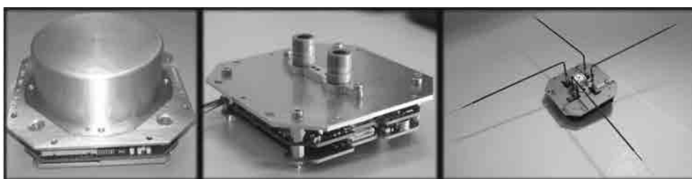
Fig.3.7 Three types of QB50 science sensors (from left to right): the Ion-Neutral Mass Spectrometer (INMS), the Flux-U-Probe Experiment (FIPEX) and the multi-Needle Langmuir Probe (m-NLP). Image Credit: The QB50 Consortium ( https://www.qb50.eu/ )
