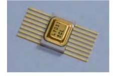
FM Low Voltage Differential Signalling Receiver & Transmitter
