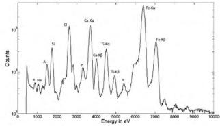
Fig 1: Left - CLASS Flight instrument. Right - Spectrum of JSC-1A with Na line demonstrating the low energy capability of CLASS. 'e' in figure means escape peak
