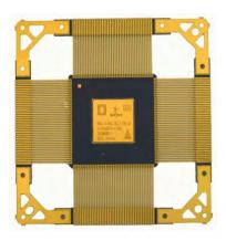
Inertial Sensor Acquisition ASIC
