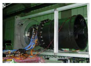
Fig.3: Carto-3 EOM integrated with Payload Electronics & FPA
