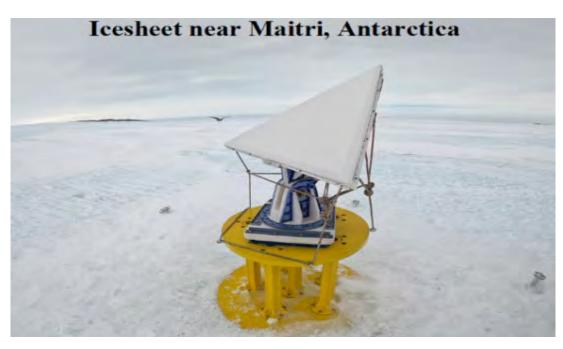
Fig 14: Corner reflectors installed at Antarctica during 39 ISEA
