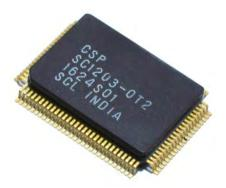
CCD Signal Processor ASIC
