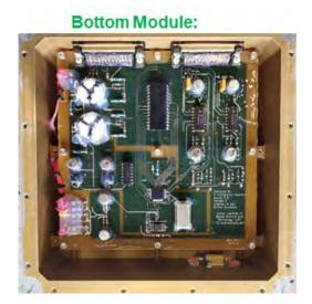
Fig 1: Different parts (top and bottom modules) of the ARIS payload, assembled with the retarding potential analyzer and associated electronic printed circuit boards
