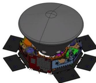
Figure 40 – SCC with deployed Solar Arrays (credit: TAS)
