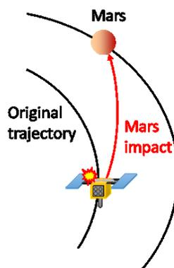
Figure 26 – Spacecraft impact on Mars on a ballistic trajectory.
