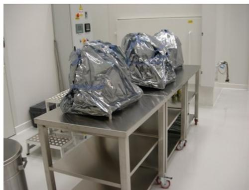
Figure 46 – Temporary biobarriers covering flight hardware placed into a bioburden controlled cleanroom at TASinI premises (credit TAS)
