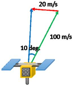
Figure 28 –  $\Delta V$  generated by guidance error.
