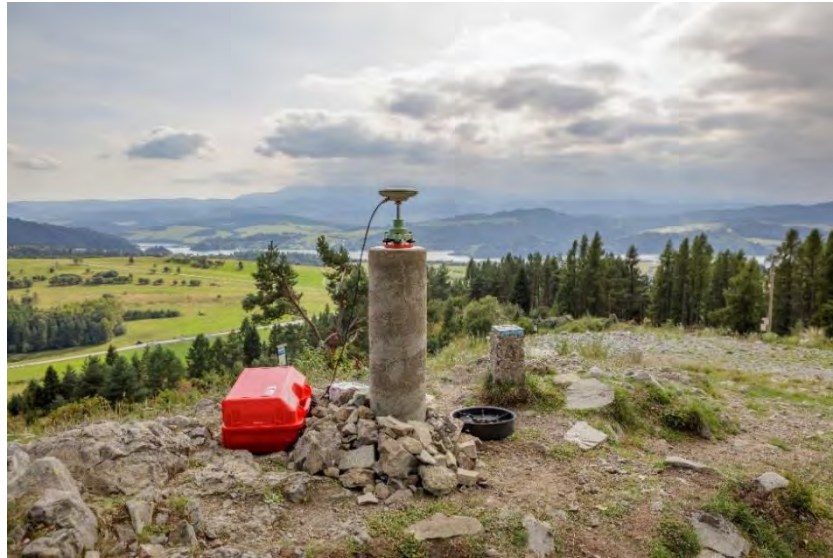
Fig. 1.39. Measurement at geodetic reference baseline [photo: M Wiśniewski, GUM].
