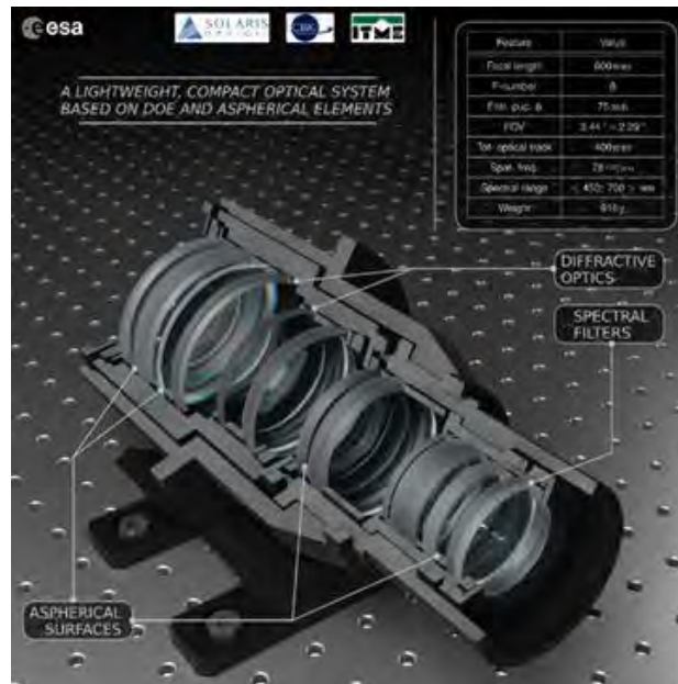
Fig. 4.19. The proposed design of the new DOE optics, © CBK PAN
