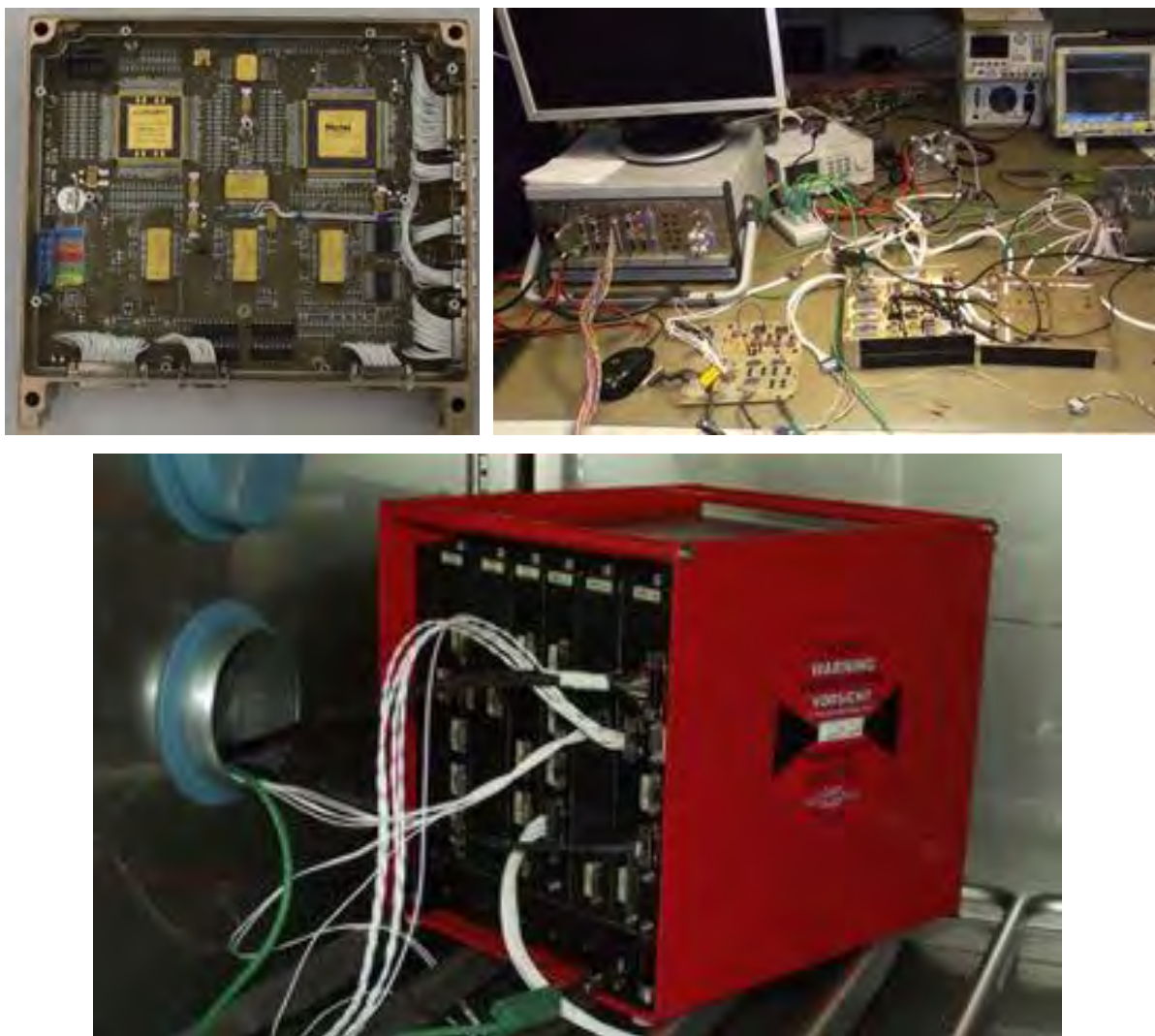
Fig. 4.14. PROBA3 CCB: DPU EQM PCB (top left), the functional tests of CCB modules (top right) and the thermal tests of integrated CCB EQM(bottom), © CBK PAN
