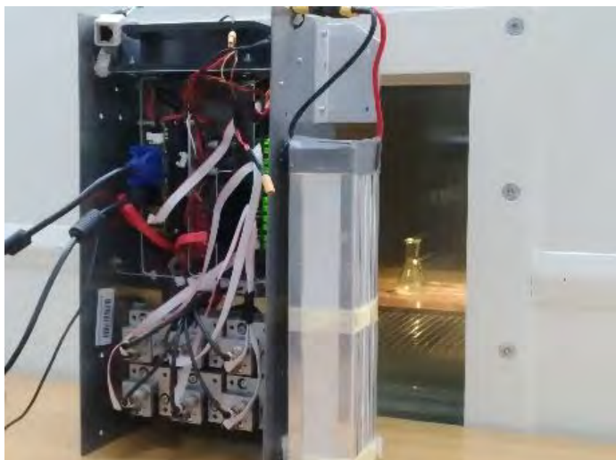
Fig. 5.2. Vacuum chamber experiment with methanogenic archaea and Enceladus' ocean analog.
