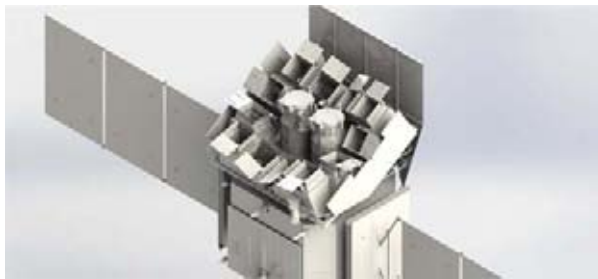
Fig. 1 Layout of the Einstein Probe spacecraft and scientific payloads, which include 12 modules of WXT aligned to mosaic the total 3600 square degrees field of view and 2 coaligned modules of FXT (credit: IMAC/CAS)
