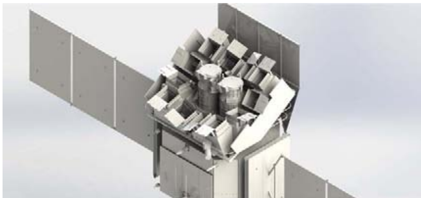
Fig. 9 Layout of the Einstein Probe spacecraft and scientific payloads, which include 12 modules of WXT aligned with different directions and 2 coaligned modules of FXT
