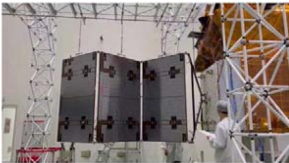
Fig. 13 Solar array deployment testing—panel unfolding (credit: IMAC)
