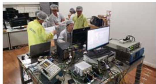
Fig. 12 Satellite to ground S-band interface compatibility test
