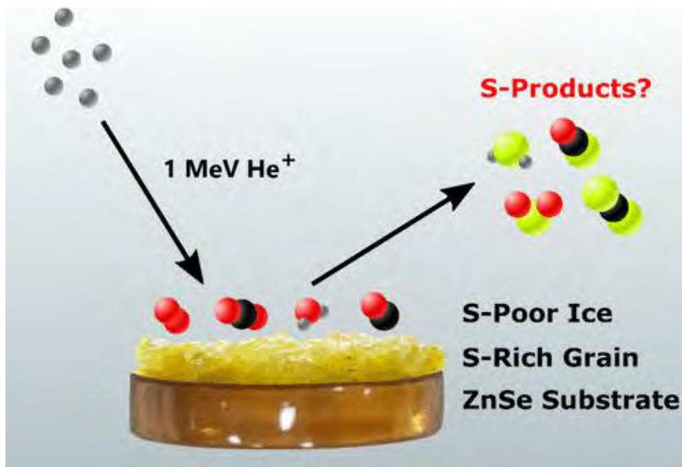
Figure 2.14. Conceptual illustration of the experimental approach used to search for sulfur-bearing molecules. An S-free ice is deposited on a layer of allotropic sulfur supported by a ZnSe substrate. Irradiation with 1 MeV He + ions simulates energetic particle processing in astrophysical environments. Energy deposition in the ice and sulfur layer may trigger chemical reactions and mixing, potentially leading to the formation of sulfur-bearing molecular products in the processed ice.
