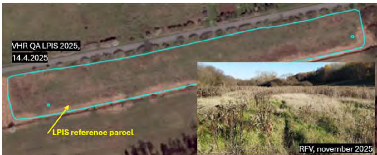
Figure 5.16. Example of identification of a potential critical defect - Total absence of eligible features on the QA VHR 2025. It was confirmed by rapid field visit. It was not a systematic error, but a mistake caused by update – changes of the underlying land were not applied (the land use change occurred after the cyclical update of LPIS).
