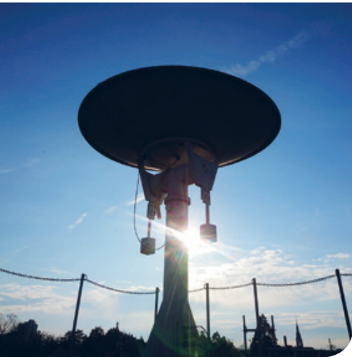
Receiving antenna at UNIBERN operated by the Remote Sensing Research Group, Institute of Geography, since August 2000. The received and archived data are the backbone of the European AVHRR Master Data-Set re-processed in the frame of the FDR4AVHRR project.
