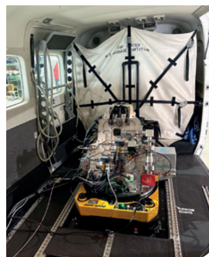
AVIRIS-4 instrument built into a Cessna Caravan operated by Swiss Flight Services.
