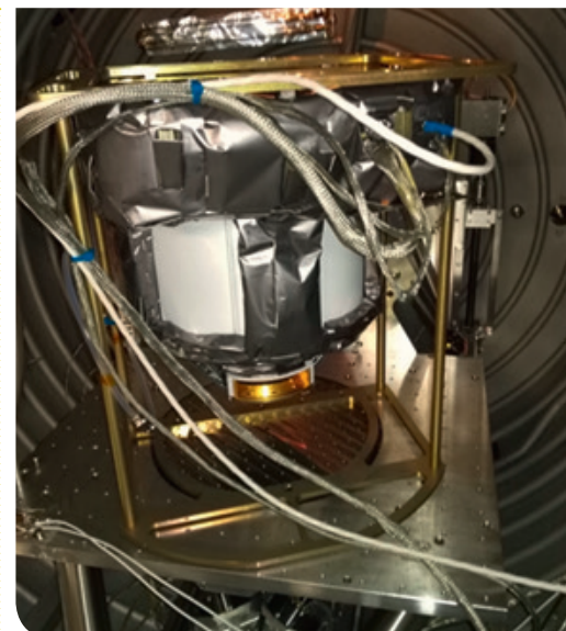
Heavy Ion Sensor (HIS) during calibration in the MEFISTO facility for highly charged ion beams at the Univ. of Bern.
