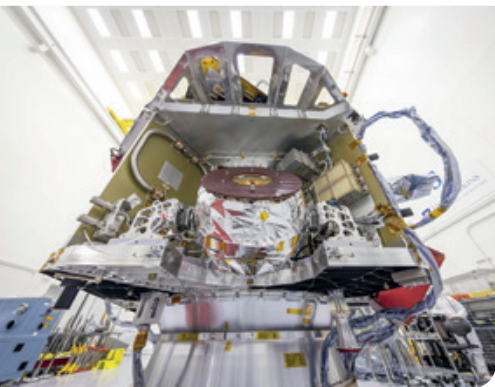
The IMAP-Lo instrument is shown installed on the Interstellar Mapping and Acceleration Probe (IMAP) at the Johns Hopkins Applied Physics Laboratory in Laurel, Maryland, USA. The IMAP-Lo entrance is covered by a red protection cover. Image Credit: NASA, Johns Hopkins APL, Princeton, Ed Whitman.
