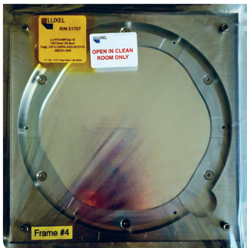
One of the full-scale X-IFU optical blocking filters procured by the UNIGE team from LUXEL (USA) during the previous Athena phase A/B1. The photo shows the complex honeycomb structure of the metallic mesh glued on the filter to support the membrane. This filter was 160 mm in clean aperture. The re-designed filters for NewAthena have an increased diameter up to 250 mm (clean aperture).
